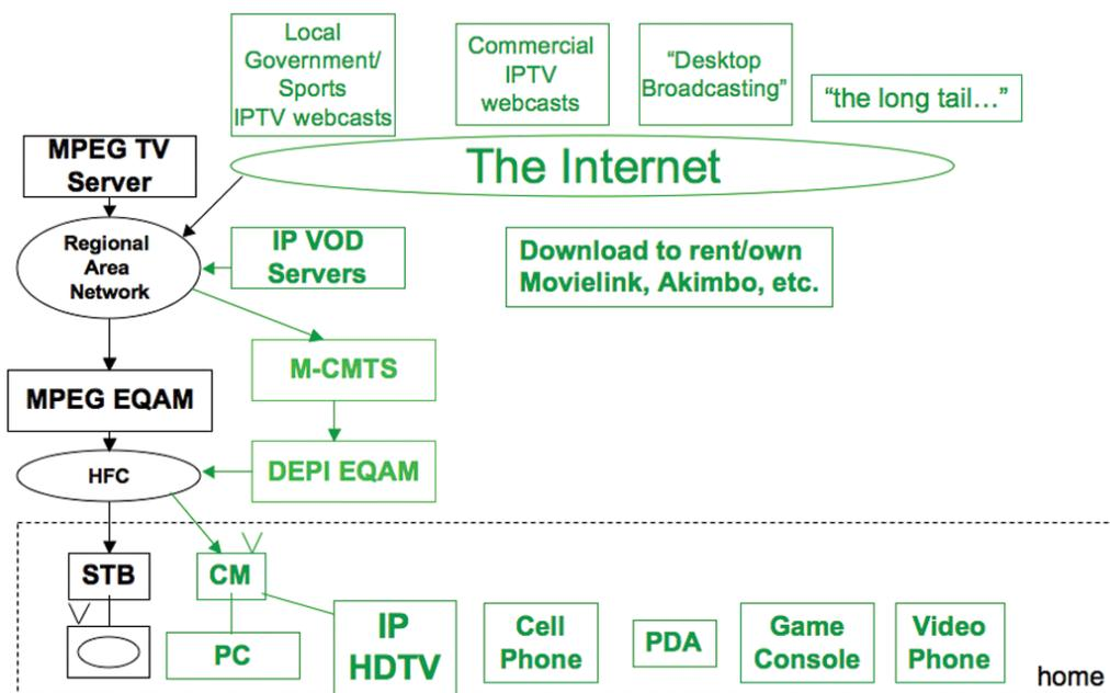
Figure 2: Internal Structure of the Cable Network<sup>16</sup>
