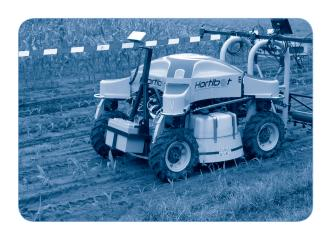
use of chemicals for weed control. Danish scientists have developed the "Hortibot," a robot that uses visual sensing to navigate crop rows and then uses either manual weed removal tools or precision herbicide spraying to kill weeds.
